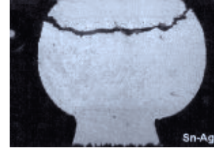
Fig. 3. Fracture of SnAg Solder Ball [13]
