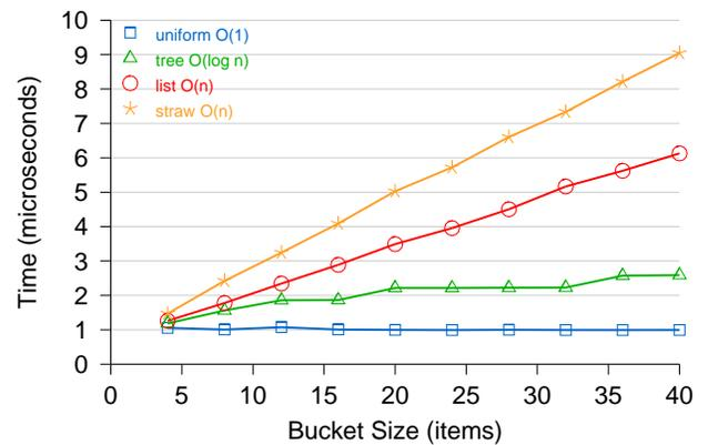
**Figure 8: Low-level speed of mapping replicas into individual CRUSH buckets versus bucket size. Uniform buckets take constant time, tree buckets take logarithmic time, and list and straw buckets take linear time.**
