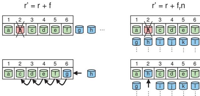
**Figure 2: Reselection behavior of *select(6,disk)* when device  $r = 2$  ( $b$ ) is rejected, where the boxes contain the CRUSH output  $\vec{R}$  of  $n = 6$  devices numbered by rank. The left shows the “first  $n$ ” approach in which device ranks of existing devices ( $c, d, e, f$ ) may shift. On the right, each rank has a probabilistically independent sequence of potential targets; here  $f_r = 1$ , and  $r' = r + f_r n = 8$  (device  $h$ ).**
