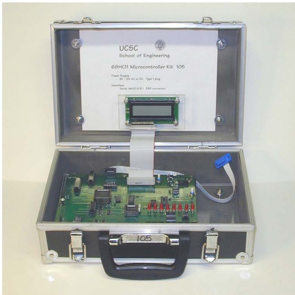
Fig.1. Finished Microkit showing significant features: LCD, slide switches, LED’s, serial interface cable with DB25 connector, and protective plastic assembly.
