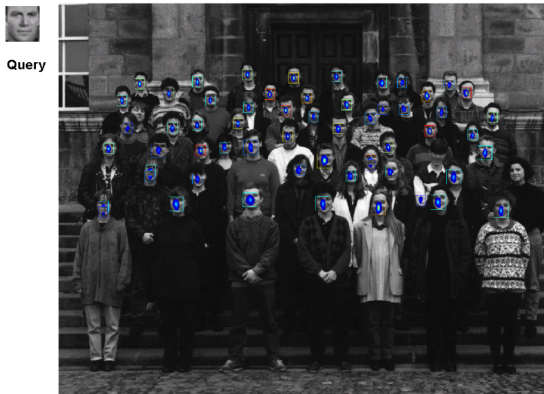
Fig. 18. Detection Results on the MIT-CMU multi-scale test set [54]. \alpha was set to 0.99. Among 57 faces present, we detected 54 faces at a correct location with 4 false alarms.
