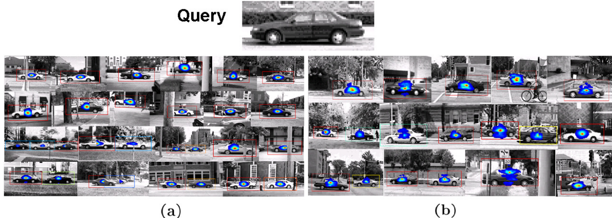
Fig. 13. (a) Examples of correct detections on the UIUC single-scale car test set [53]. (b) Examples of correct detections on the UIUC multi-scale car test set. Confidence level \alpha was set to 0.99 and RM only above the threshold \tau corresponding to \alpha is embedded in test images. Bounding boxes are drawn at the correct locations. In case of a multiple detection, a red bounding box indicates higher resemblance to Query than a blue bounding box.
