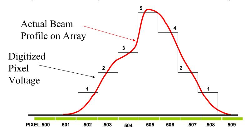
Voltage array  $X = \{0, 0, 0, 0, 0, \dots 0, 0, 0, 0, 0, 1, 2, 3, 5, 4, 2, 1, 0, 0, 0, 0, 0, 0, \dots 0, 0, 0, 0, 0, 0, 0, 0, 0\}$  2048 values
