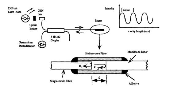
Figure 4. Extrinsic Fabry-Perot interferometric fiber sensor.
