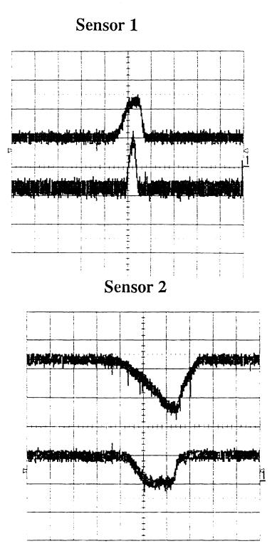
Figure 7. EFPI output under loading conditions, showing successful connectorization of embedded fiber sensors, a) EFPI output during bending through connector 1 and b) EFPI output from connector 2. Both oscilloscope traces are 1 volt/div vertical scale and 1 sec/div horizontal scale.
