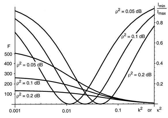
Figure 4. Finesse and Minimum Dip Intensity as a Function of Splitting Ratio.
