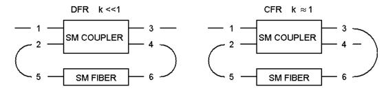
Figure 3. DFR and CFR Topology Examples.
