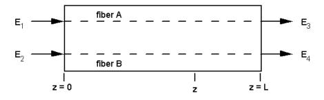
Figure 1. 2×2 Coupler Block Diagram.
