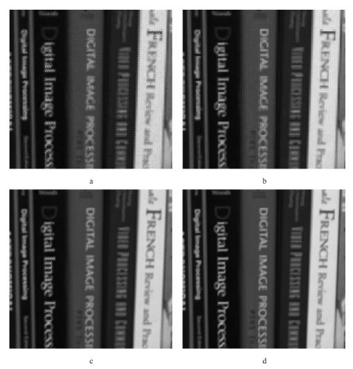
Fig. 13. Multiframe color super-resolution implemented on a real data sequence. (a) One of the input LR images demosaiced by [14] and (b) one of the input LR images demosaiced by the more sophisticated [16]. (c) Result of applying the proposed color-super-resolution method on 31 LR images each demosaiced by [14] method. (d) Result of applying the proposed color-super-resolution method on 31 LR images each demosaiced by [16] method.
