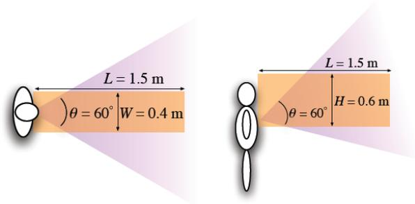
Fig. 1: Illustration of the placement of the described ETA. The coverage area of the typical ultrasound sensor (purple) is shown along with the ideal hazard detection area (orange).
