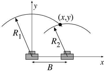
Fig. 3: The geometry of bilateration.
