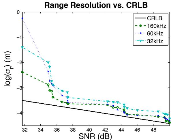
Fig. 4: Range estimation performance of our laboratory prototype utilizing a 1000  $\mu$ s Barker encoded sinusoid (length 5 code with a sinusoid center frequency of 40 kHz). The Cramer-Rao Lower Bound (CRLB) and the standard deviation of range estimates for several different sampling frequencies (red: 160 kHz; green: 60 kHz; blue: 32 kHz) are plotted against the SNR. Note that the test system is capable of sub-millimeter range resolution.
