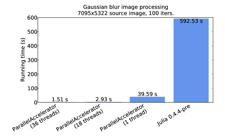
Data from 03/02/2016 2 Intel(R) Xeon(R) CPU E5-2699 v3 @ 2.3GHz processors, 18 cores each (36 cores total) 128 GB RAM
