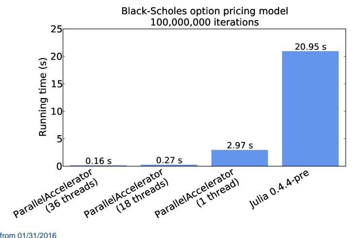
Data from 01/31/2016 2 Intel(R) Xeon(R) CPU E5-2699 v3 @ 2.3GHz processors, 18 cores each (36 cores total) 128 GB RAM
