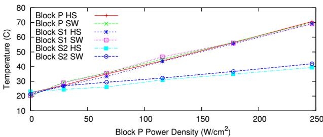
Fig. 4. Temperatures for blocks P, S1, and S2 with different constant power in block P. HS and SW stand for AMD Mobile heat sink and sapphire window respectively.
