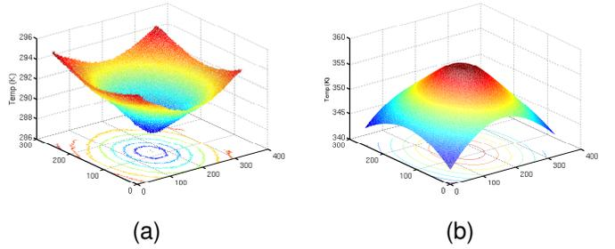
Fig. 3. (a) IR Measured temperature with low and (b) high temperature behavior for IR camera. (Temperature scale in Kelvin)
