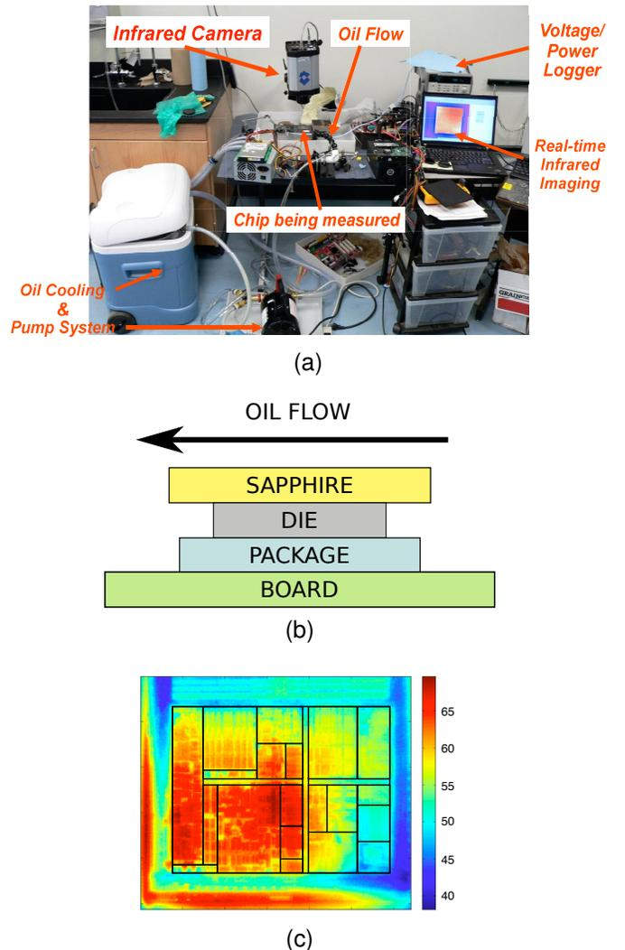
Fig. 1. (a) Measuring setup; (b) Oil-based heatsink with laminar flow, (c) a snapshot of a device with floorplan mapped on it (Temperature in Celsius).
