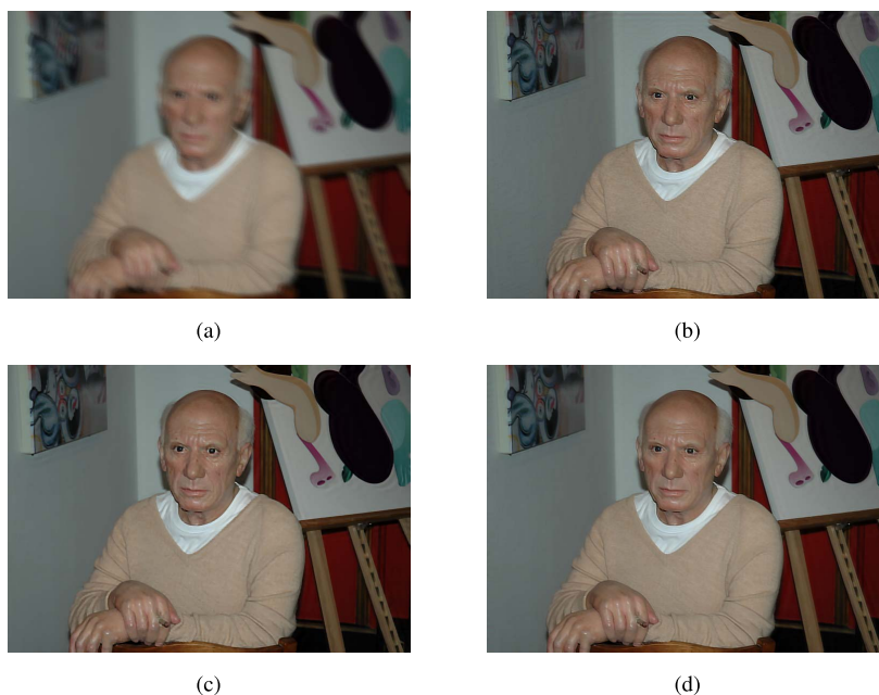
Fig. 13. Real motion deblurring example: (a) input blurred noisy image, (b) Output of hyper-Laplacian algorithm [20], (c) output of [22], and (d) output of our algorithm ( \eta = 0.031 , \beta = 0.6 ).
