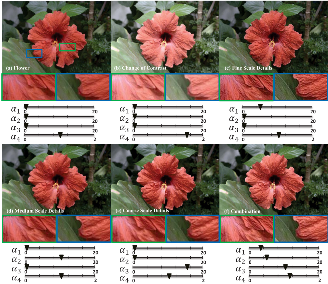
Fig. 8. Contrast and detail manipulation of the flower image. (a) Input image, (b) \alpha_1 = 1, \alpha_2 = 1, \alpha_3 = 1, \alpha_4 = 1.5 , (c) \alpha_1 = 5, \alpha_2 = 1, \alpha_3 = 1, \alpha_4 = 1 , (d) \alpha_1 = 1, \alpha_2 = 10, \alpha_3 = 1, \alpha_4 = 1 , (e) \alpha_1 = 1, \alpha_2 = 1, \alpha_3 = 15, \alpha_4 = 1 , (f) \alpha_1 = 3, \alpha_2 = 5, \alpha_3 = 10, \alpha_4 = 1.1 .
