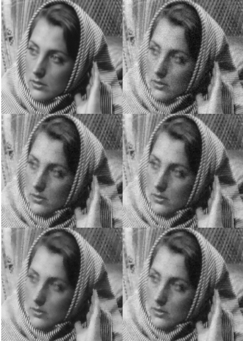
Figure 4.6: Enlarged region of denoised image. From left to right and top to bottom: Original image, Tikhonov, TV, B-TV Multiscale L-G mixture, single scale L-G mixture
