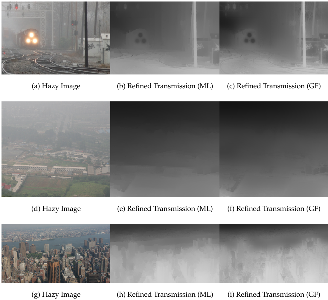
Figure 3.4: Comparison between results of the Matting Laplacian(ML) and Guided Filter(GF) for various images. Matting Laplacian parameters are \epsilon = 10^{-4} , and \lambda = 10^{-3} . Guided Filter parameters are \epsilon = 10^{-2} , and r = 30
