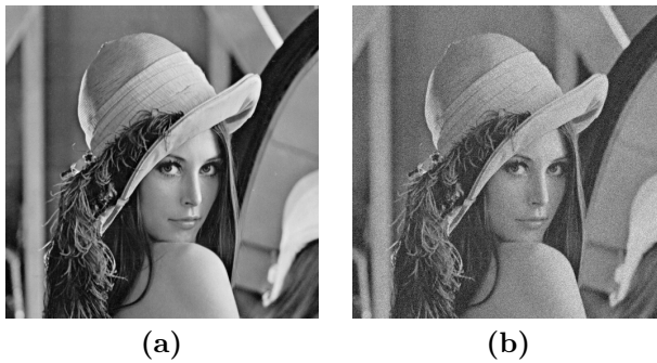
Figure 6.3: (a) The original 'Lena' image (b) 'Lena' with added white Gaussian noise of variance 229 (MSE= 229.0)
