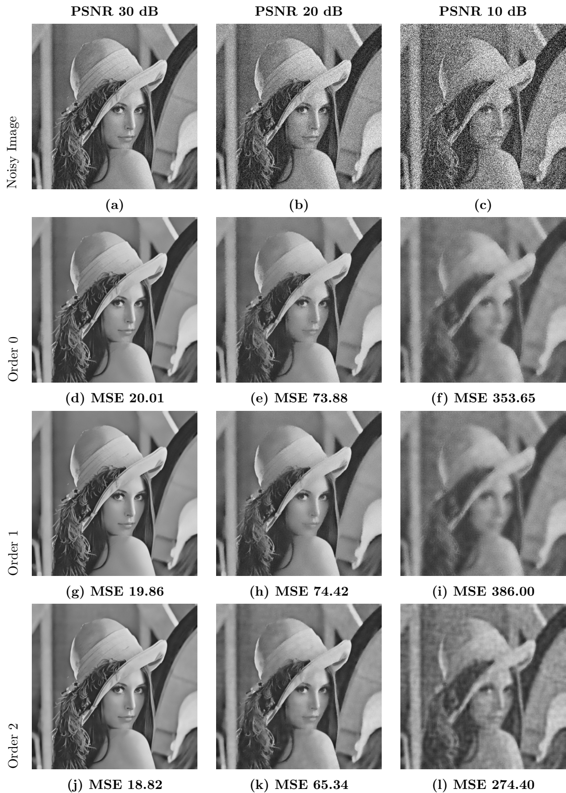
Figure 3. Results of denoising using NLM method of orders 0, 1 & 2. The MSE values reported are the average MSE of the denoised results obtained over simulations with 20 different realizations of zero mean Gaussian noise in each PSNR case.
