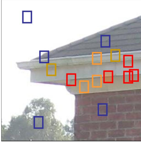
Figure 1. An image showing similar and dissimilar patches. The patch under consideration is the shaded red patch. Other red patches are similar and hence contribute more to denoising of the pixel at the center of the shaded patch. The blue patches are totally dissimilar and hence are ignored. The orange patches bear some resemblance but are not totally similar and hence their contributing weights are lesser than the red patches.
